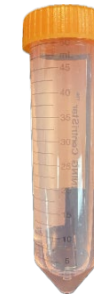
50 ml dilution medium vial Must be kept refrigerated until 1 hour prior to use.
